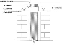
10. Using a knife or hacksaw, trim the liner to within 1" of the chimney flashing. Secure the Rain Cap to the liner with three evenly spaced screws (provided).
