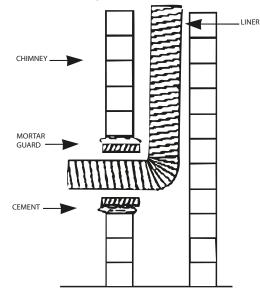
12. Trim the liner at the bottom with a knife or hacksaw and attach the chimney connector pipe into the liner.
