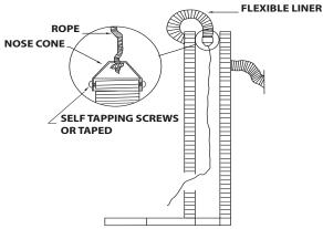
9. Allow at least 6 inches to 12 inches of the liner to extend above the top of the chimney for attaching Rain Cap. Place the chimney flashing over the liner and secure to chimney using nail-in anchors. Caulk all joints with a quality silicone sealant and paint if required.
