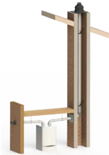
Vertical Flex Vent in Clean Unused Chimney with Chimney Cover and Horizontal Air
