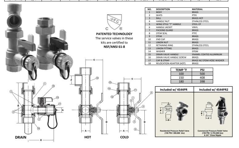
**Specifications:** Designed for residential or commercial use with potable water. This approved Webstone valve is actuated by a blowout proof stem and features an adjustable packing gland. Threaded ends comply with ANSI B1.20.1.
