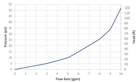
Tolerance is within  $\pm$  10%. Max flow is 8 gpm when set temp above 125 F
