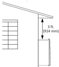
Do not install the water heater vent terminator within 1 ft. (305 mm) in the USA of any air intake or building opening, and within 3 ft. (914 mm) in Canada of any air intake or building opening (Outdoor models only, refer to p. 22).
