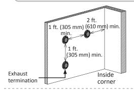
For multiple sidewall exhaust terminations (e.g. Multi-Unit Systems), an exhaust termination must be at least 1 ft. (305mm) away from another exhaust termination. An exhaust termination must also be at least 2 ft. (610 mm) away from an inside corner. (If the adjacent wall is less than 2 ft. (610 mm) of length, the minimum required distance away from the inside corner will be equal to the length of that adjacent wall.)
