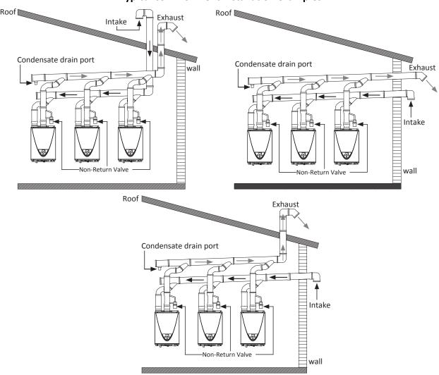
For details on the installation of a common-vent system, please refer to the vent manufacturer's instructions.
