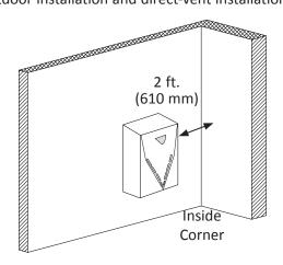
Do not install next to a dryer or any source of airborne debris that can be trapped inside the combustion chamber, unless the system is direct-vented.
