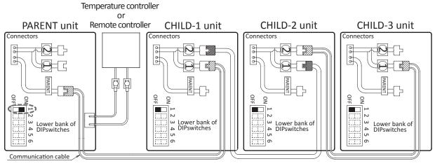
**NOTE:** The dark squares indicate the direction the DIPswitches should be set to.
