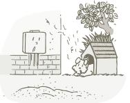
Do not have the vent terminal pointing toward any opening into a building. Do not locate your heater in a pit or location where gas and water can accumulate.
