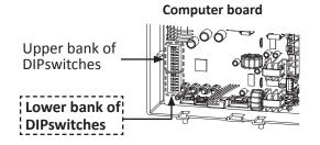
**NOTE:** Only change the switches with dark squares. The dark squares indicate the direction the DIPswitches should be set to.
