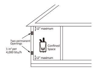
Figure 2 - Direct to outdoors openings Two permanent openings
