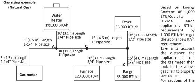
Content of 1,000 BTU/Cubic ft: each appliance's BTU/h requirement by 1,000 BTU/ft<sup>3</sup> to get the appliance's ft<sup>3</sup>/h requirement. Take into account the distance the the gas meter, then look in the above gas chart to properly size the line. For sections of the
