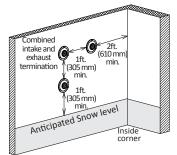
For multiple-unit, direct-vent sidewall terminations that combine the intake and exhaust into a single penetration, space each direct-vent termination at least 1 ft. (305 mm) away from each other, no matter the orientation. A directvent termination must also be at least 2 ft. (610 mm) away from an inside corner. If the adjacent wall is less than 2 ft. (610 mm) of length, the minimum required distance away from the inside corner will be equal to the length of that adjacent wall.
