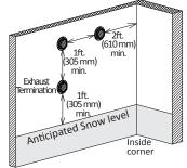
For multiple sidewall exhaust terminations (e.g. multiunit systems), an exhaust termination must be at least 1 ft. (305mm) away from another exhaust termination. An exhaust termination must also be at least 2 ft. (610 mm) away from an inside corner. If the adjacent wall is less than 2 ft. (610 mm) of length, the minimum required distance away from the inside corner will be equal to the length of that adjacent wall.
