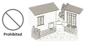
Do not install the water heater direct vent terminator within 1 ft. (30 cm) in the USA of any air intake or building opening, and within 3 ft. (91 cm) in Canada of any air intake or building opening ( Refer to pp. 24 and 25.).
