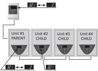
9009069005 (TM-RE42) **Outdoor model installation** 321 ↔ 2 • Unit #2: The green LED on the computer board will be flashing twice, just like in the single unit example. • Unit #3 and #4: Unit #1 Unit #2 Unit #3 Unit #4 The green LED on the computer board will stay off. PARENT CHILD CHILD CHILD 321
