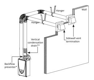
\*Backflow preventer (Recommended for freezing weather conditions: 36 °F (2 °C) and below).
