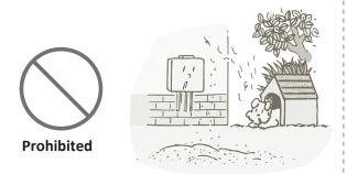
Do not install this water heater under an overhang less than 3 ft. (914 mm) from its top or eaves. The area under an overhang must be open to three sides (Outdoor models only).
