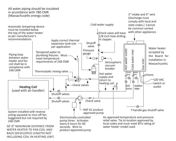
The recirculation pump is to provide no less than 2 GPM (7.5 L/min) and no more than 4 GPM (15 L/min) through each activated unit in the system
