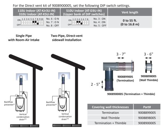
\*Backflow preventer (Recommended for freezing weather conditions: 36 °F (2 °C) and below.)
