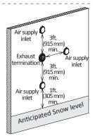
For direct-vent sidewall terminations that use two separate penetrations for the intake and exhaust, distance the intake and exhaust terminations at least 3 ft. (915 mm) away from each other, no matter the orientation unless they follow case 1 and 2 on p. 23.
