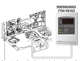
Connect other end to these terminals Front of remote Fig. E-2
