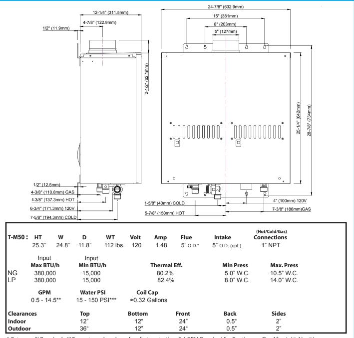
\* Category III Required \*\*Current numbers based on factory testing, 0.4 GPM Required for Continuous Fire After initial Ignition. \*\*\*Pressure Only Relief Valve Requires (Min. 380,000 BTUs. 150 PSI). Min 40 PSI or above recommended for maximum flow.
