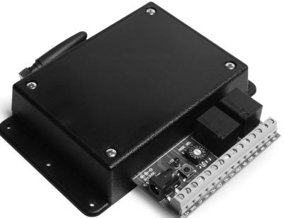
The input voltage is not to exceed 20 volts.
