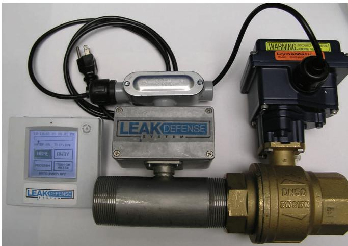
The LDS-002-150 is an electronic water flow monitor and alarm system designed to detect leaks in 2" water pipes, in plumbing fixtures and in water using appliances. An alarm is triggered if continuous water flow exceeds the preset time limit. If this occurs, an audible alarm will sound and the water supply will be shut-off, potentially preventing major water damage. This unit includes a brass motorized ball valve and the Sentinel Hydrosolutions Residential Control Panel.
