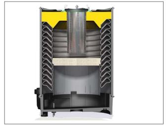
Fig. 7 Heat exchanger & Burner cross-sectional view
