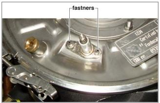
Fig. 79 Electrode fasteners
