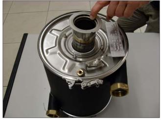
Fig. 6 Burner head
