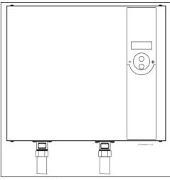
Fig. 6 Vertical mounting position
