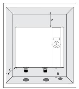
Fig. 5 Recommended minimum clearances
