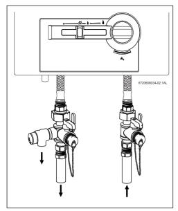
Fig. 15 Plumbing connections and pressure relief valve shown with optional Webstone service valves
