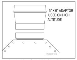
Fig. 10 Vent Adaptor for High Altitude Installations
