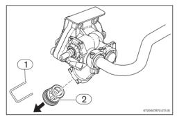
Fig. 25 Drain plug and filter location
