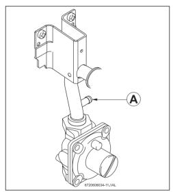
Fig. 14 Gas pressure measuring point
