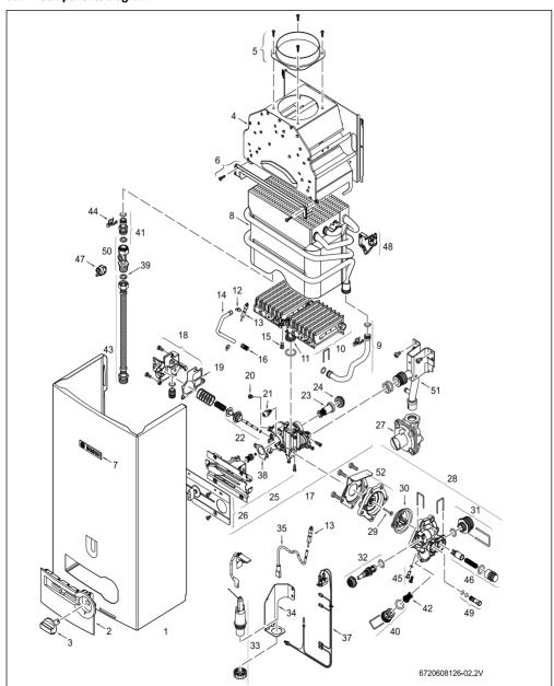
Fig. 28 Components Diagram
