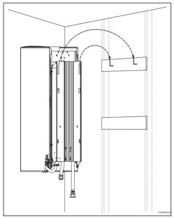
Fig. 8 Secure heater to wall
