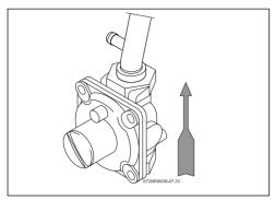
Fig. 13 Installation of Gas Pressure Regulator
