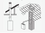
Venting into a masonry chimney with approved liner, ceramic tile, clay or metal is permissible. For complete venting options and requirements, download the Product Manual at **www.boschheatingandcooling.com**
