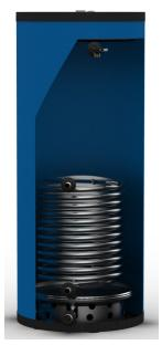
tendencies of domestic water. The tanks feature a high capacity stainless steel coil that efficiently transfers BTU's from the heat source to domestic water stored in the tank, making 1st hour delivery among the industry's best. Two-inch thick, highdensity insulating foam with a tested R value of 13.4. surround the tank for low stand by losses. The SST series offer tank capacities 40, 65, 80 and 113 gallons to suit all your hot water needs.
