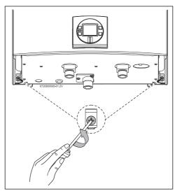
Fig. 3 Loosen the two screws
