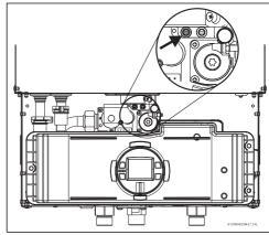
Fig. 38 Gas pressure test port (left tapping)
