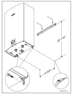
Fig. 30 Mounting the heater in manufactured (mobile) homes
