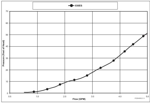
Fig. 36 Pressure drop curve
