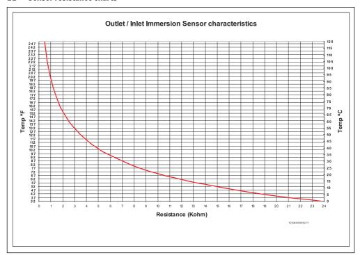
Fig. 64 Outlet / Inlet immersion sensor characteristics
