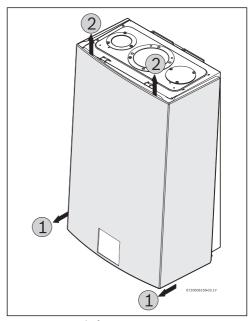
Fig. 4 Remove the front cover
