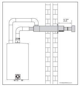
Fig. 15 Horizontal venting system (concentric vent)
