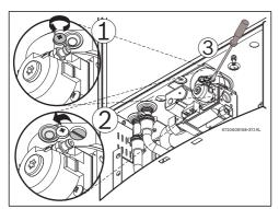
Fig. 61 Adjusting P1 CO<sub>2</sub> level
