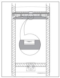
Fig. 28 Leveling wall mounting bracket
