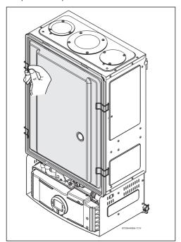
Fig. 5 Remove the combustion cover
