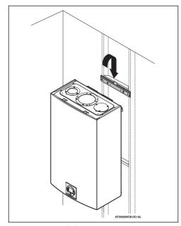
Fig. 29 Mounting the heater
