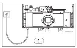
Fig. 39 Connecting power supply cord
