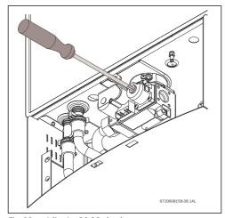
Fig. 62 Adjusting P2 CO<sub>2</sub> level
