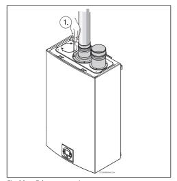
Fig. 20 Exhaust connection
