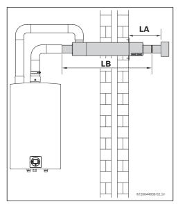
Fig. 10 Concentric kit installation
