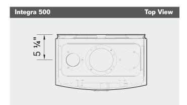
Note: Intake can be installed on the left or right side of the exhaust.
