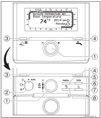
Fig. 57 FW 200 heating control with front flap closed / flap opened
