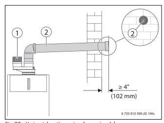
Fig. 33 Horizontal venting system (room air only)
