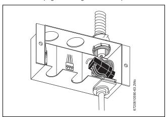
Fig. 45 Cable connected (external pump)
