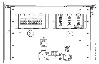
Fig. 42 Installer junction boxes with covers removed
