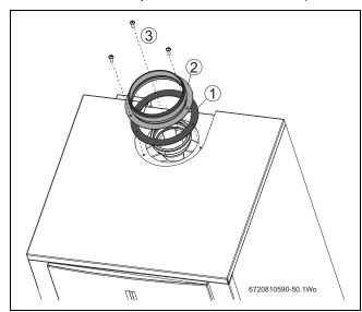
Fig. 26 Attaching the vent flange and gasket
