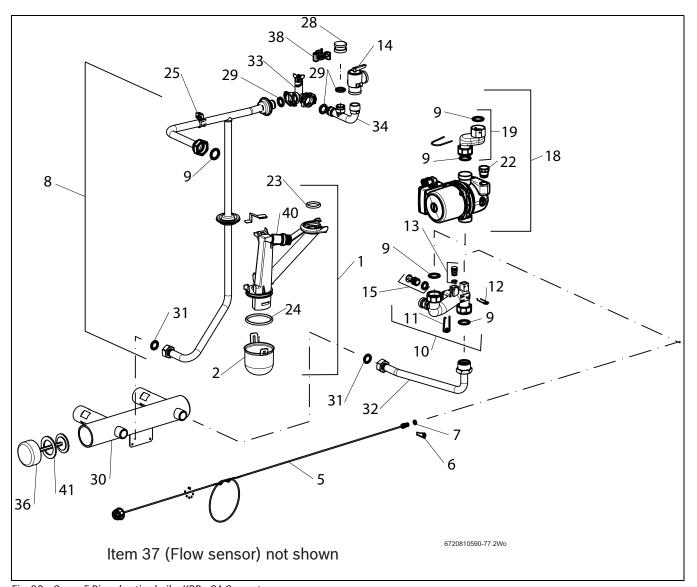
Fig. 98 Group 5 Pipes heating boiler KBR.. 3A Greenstar
