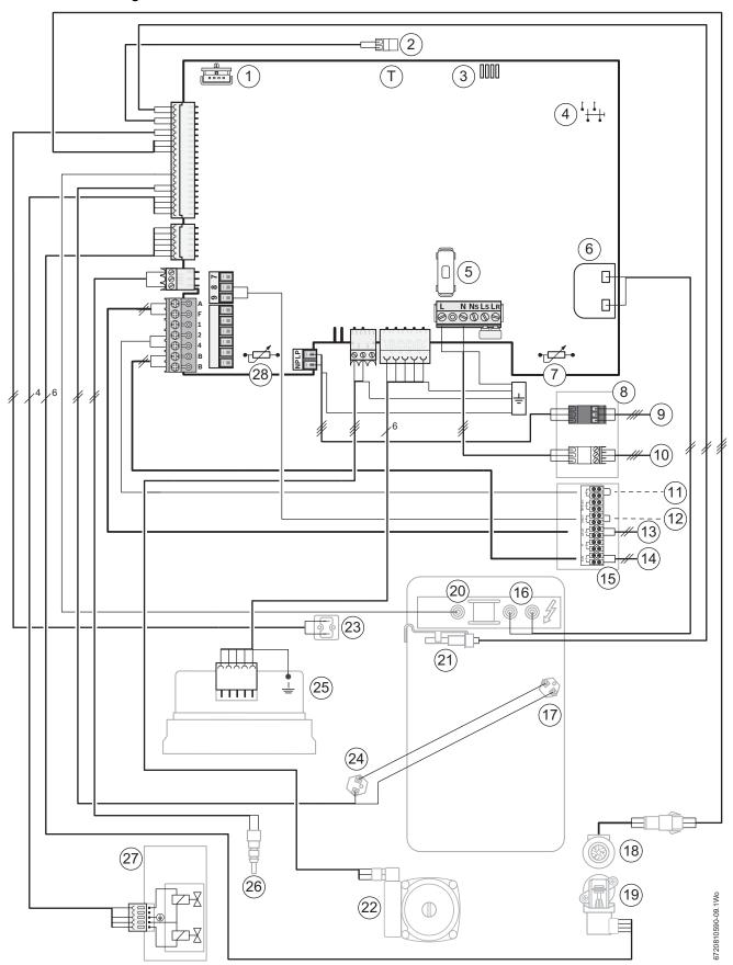
Fig. 9 Electrical wiring diagram combi boiler KWB..-3A
