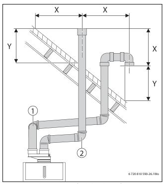
Fig. 39 Vertical venting system (sealed combustion)
