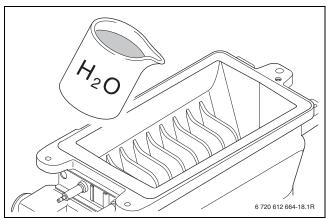
Fig. 90 Rinsing the heat exchanger
