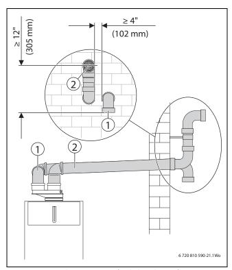
Fig. 34 Horizontal venting system (sealed combustion)
