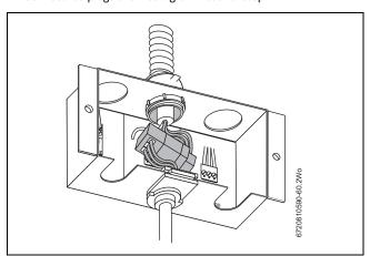
Fig. 47 Cable connected (external DHW tank loading pump or 3-way valve)
