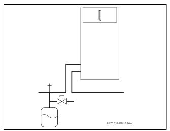
Fig. 18 Sample installation - expansion vessel
