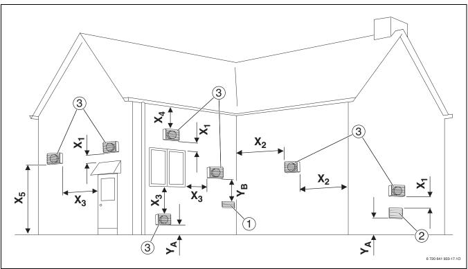
Fig. 31 Vent and combustion air pipe position
