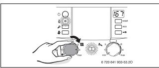
Fig. 56 Switch on heat
