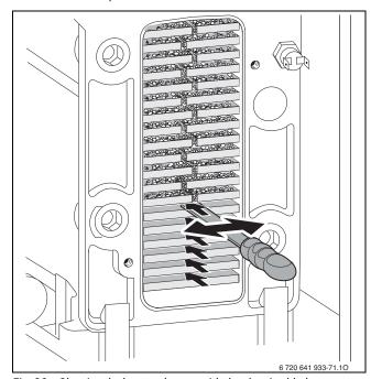
Fig. 88 Cleaning the heat exchanger with the cleaning blade
