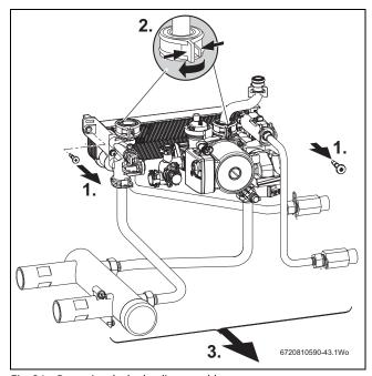
Fig. 81 Removing the hydraulic assembly
