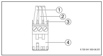
Fig. 48 Attach plug (mains power supply)
