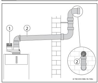
Fig. 32 Horizontal venting system (room air only)
