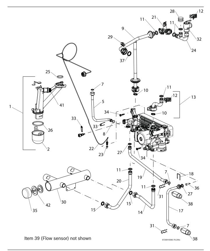
Fig. 97 Group 4 - Pipes combi boiler KWB..3A Greenstar
