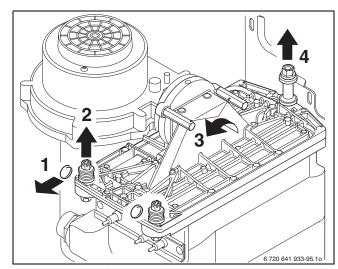
Fig. 85 Removing the burner cover
