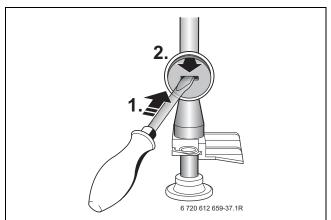
Fig. 72 Remove seal from the gas throttle
