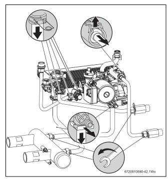
Fig. 79 Removing pipe connections
