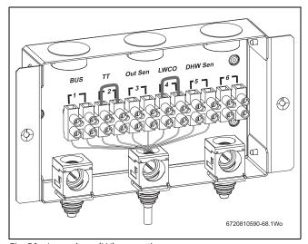
Fig. 50 Low voltage (LV) connections
