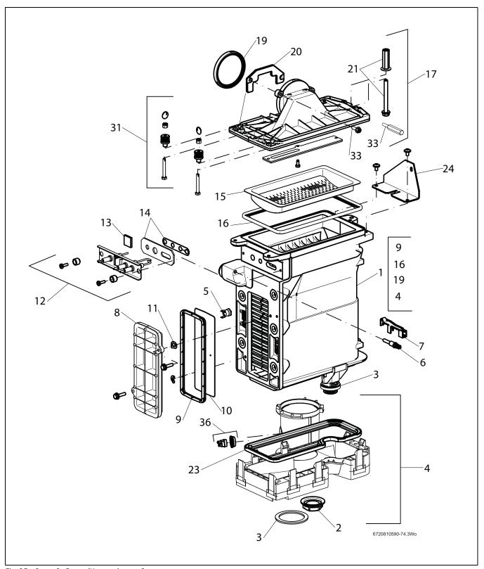
Fig. 95 Group 2 - Burner/Heat exchanger Greenstar
