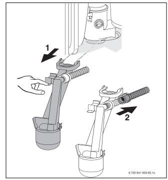
Fig. 92 Removing the condensate trap
