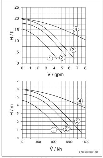
Fig. 67 Pump curve of the boiler pump combi boiler KWB..-3A
