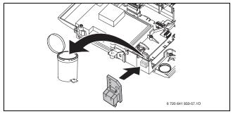
Fig. 69 Replacing the code plug
