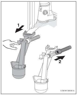
Fig. 87 Removing the condensate trap
