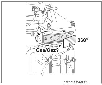
Fig. 84 Check for gas leaks
