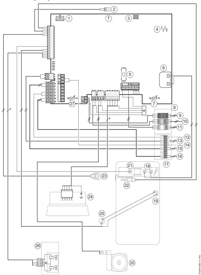
Fig. 8 Electrical wiring diagram heating boiler KBR..-3A
