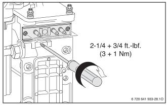
Fig. 83 Reinstalling the electrode set
