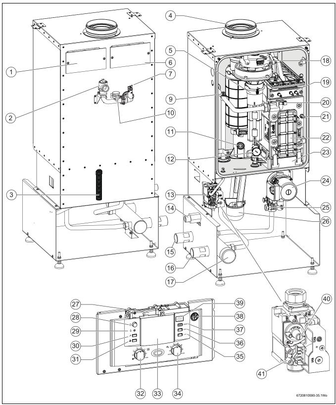
Fig. 6 Appliance layout heating boiler KBR..-3A
