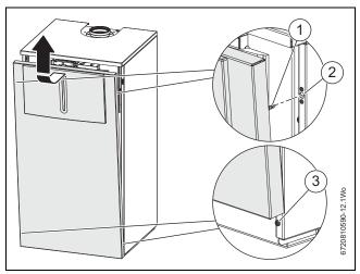
Fig. 21 Remove the cover
