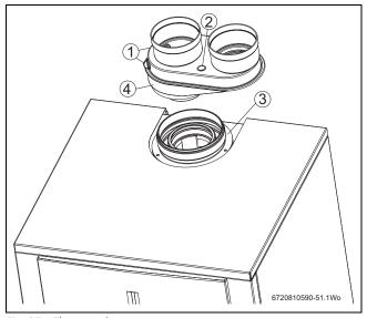
Fig. 27 Flue gas adapter
