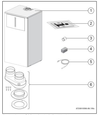
Fig. 1 Scope of delivery heating boiler KBR..-3A
