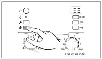
Fig. 76 Press the emissions test button
