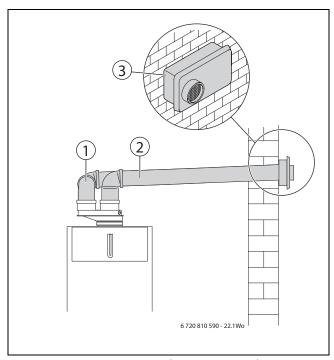
Fig. 35 Horizontal venting system (sealed combustion)
