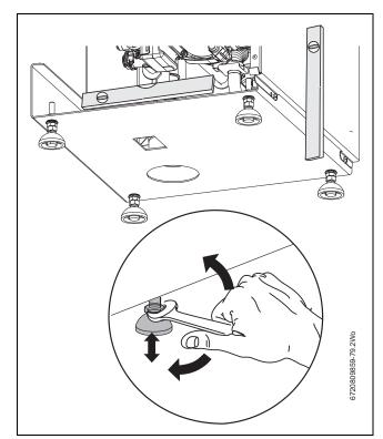
Fig. 22 Levelling the boiler
