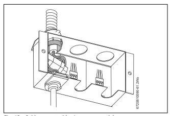
Fig. 49 Cable connected (mains power supply)
