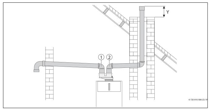
Fig. 36 Vertical venting system (sealed combustion)
