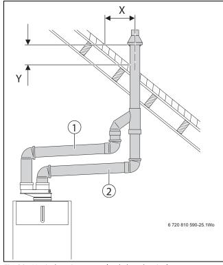
Fig. 38 Vertical venting system (sealed combustion)
