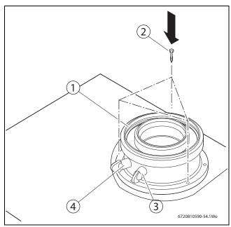
Fig. 29 Installing the concentric vent adaptor
