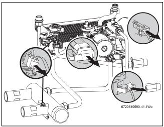
Fig. 78 Unplugging electrical connections / removing hose from PRV
