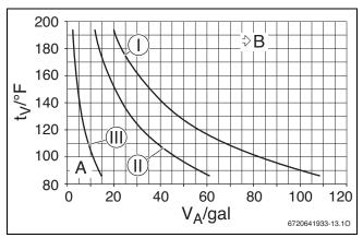
Fig. 16 Operating capacity of the expansion vessel in °F and gallons
