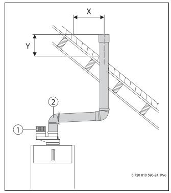
Fig. 37 Vertical venting system (room air only)
