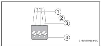
Fig. 46 Attach plug (external DHW tank loading pump or 3-way valve)
