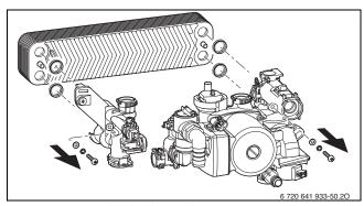
Fig. 82 Removing the plate heat exchanger
