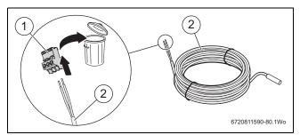
Fig. 52 DHW tank sensor connector plug removal
