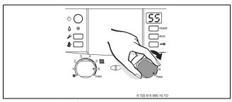
Fig. 65 Thermal disinfection
