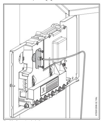
Fig. 80 Removing the boiler pressure gauge
