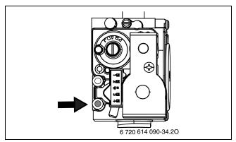
Fig. 75 Dynamic gas pressure test port
