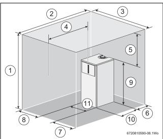
Fig. 5 Dimensions and minimum clearances (front, rear, & side view)
