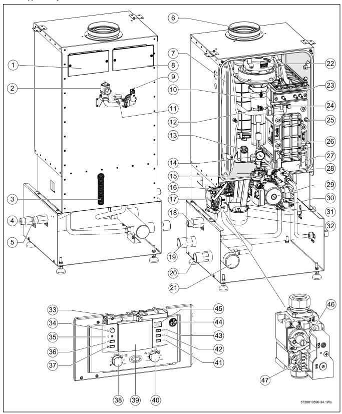
Fig. 7 Appliance layout combi boiler KWB..-3A
