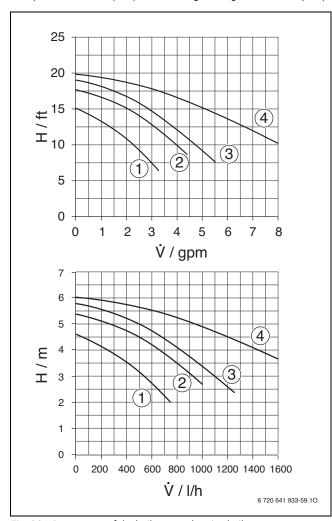
Fig. 66 Pump curve of the boiler pump heating boiler KBR..-3A
