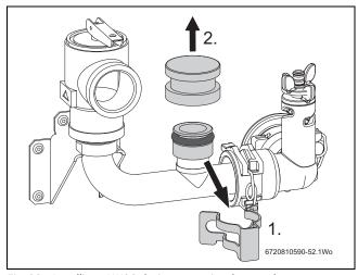
Fig. 23 Installing a LWCO device - removing dummy plug
