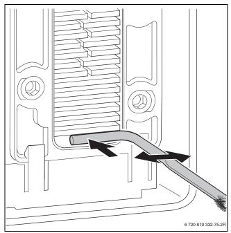
Fig. 91 Cleaning the condensate tray
