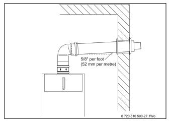
Fig. 41 Horizontal venting system (telescopic concentric vent kit)
