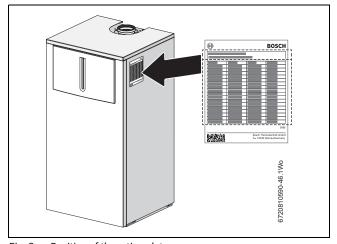
Fig. 3 Position of the rating plate
