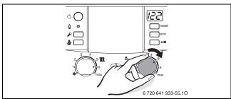
Fig. 60 Set the DHW temperature (combi boiler KWB..-3A)
