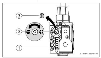
Fig. 74 Set CO<sub>2</sub> or O<sub>2</sub> level for minimum nominal output
