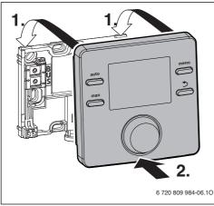
Fig. 8 Attaching the user interface
