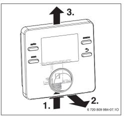
Fig. 9 Removing the user interface
