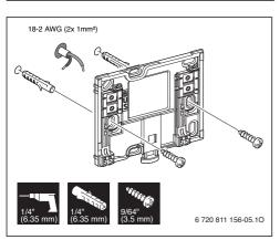
Fig. 6 Mounting the base
