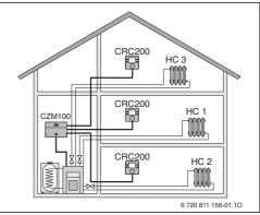
Fig. 2 Example of a heating system with three heating zones with one CZM100 and one CRC200 per zone as the controller.
