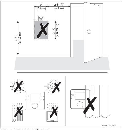
Fig. 5 Installation location in the reference room
