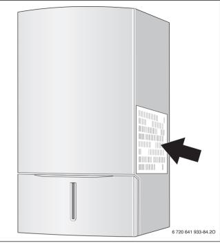
Fig. 3 Position of the rating plate
