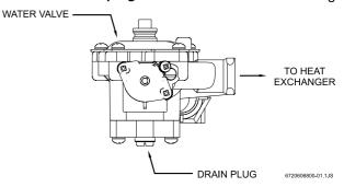
Fig. 1 - Water heater drain plug
