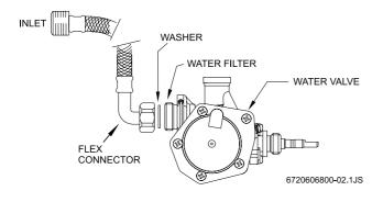
Fig. 6 - Water valve - top view
