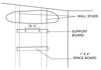
Fig. 2 - Mounting the Heater
