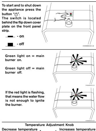
Fig. 9 - Principles of Operation
