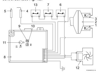
Fig. 13 - Electrical wiring diagram
