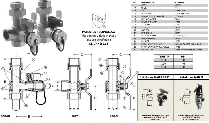
**Specifications:** Designed for residential or commercial use with potable water. This approved Webstone valve is actuated by a blowout proof stem and features an adjustable packing gland. Threaded ends comply with ANSI B1.20.1.
