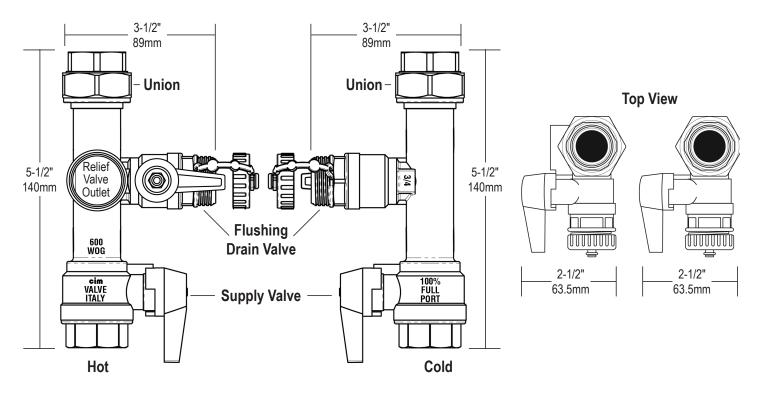
All valve kits include integrated union adapters for direct connection to cold water inlet and hot water outlet of the tankless water heater. Valve kits include integrated full port supply valves and full port system flushing/drain valves with linked cap. \*Hot water valve assembly includes outlet access port for pressure relief valve.
