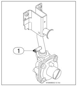
Fig. 14 Gas pressure measuring point
