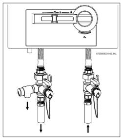
Fig. 15 Plumbing connections and pressure relief valve
